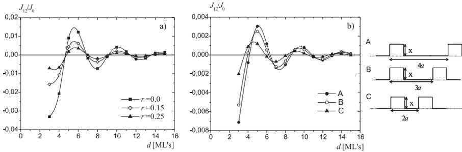
Fig. 1: The influence of a) roughness parameter  $r$  and b) roughness distribution in the interface on the interlayer exchange coupling in the function of spacer thickness  $d$ .  $r$  equal to 0 denotes the flat interface. Increasing of this value is related to a rougher interface.
