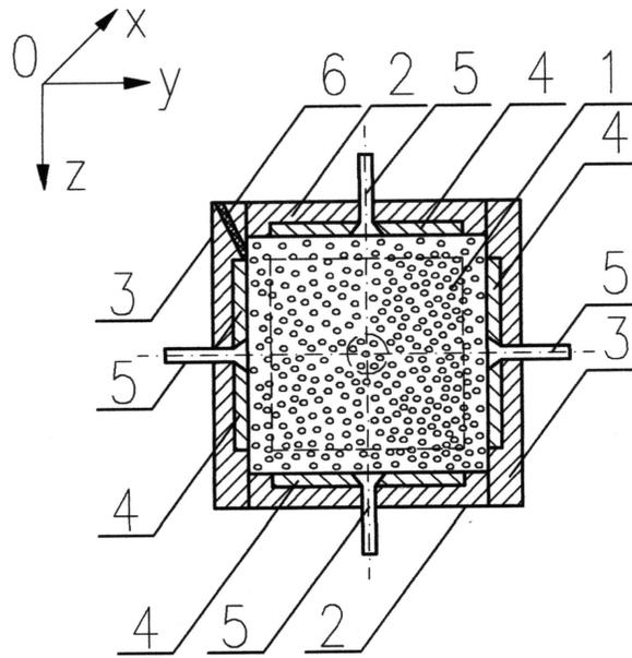
Fig. 2: Cross section of a container with a sample; 1 – magnetorheological suspension, 2, 3 – walls of the container, respectively: vertical and horizontal, 4 – electrode, 5 – lead of the electrode, 6 – canal.
