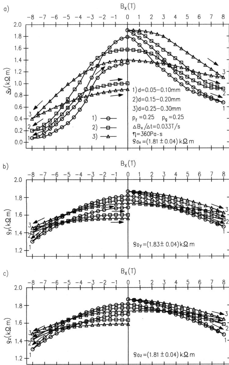
Fig. 8: Dependence of the specific resistance of the suspension sample  $\rho_x$ ,  $\rho_y$ ,  $\rho_z$  measured respectively: in directions of an  $x$ ,  $y$ ,  $z$  axis on the magnetic field induction  $B_x$ , applied along the  $x$  axis, for different sizes of iron particles  $d$ .
