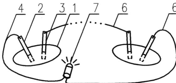
Fig. 1: The example of vegetable battery; 1 – cucumber, 2, 3 – electrodes made of different metals, 4-6 – wires, 7 – light emitting diode (LED).
