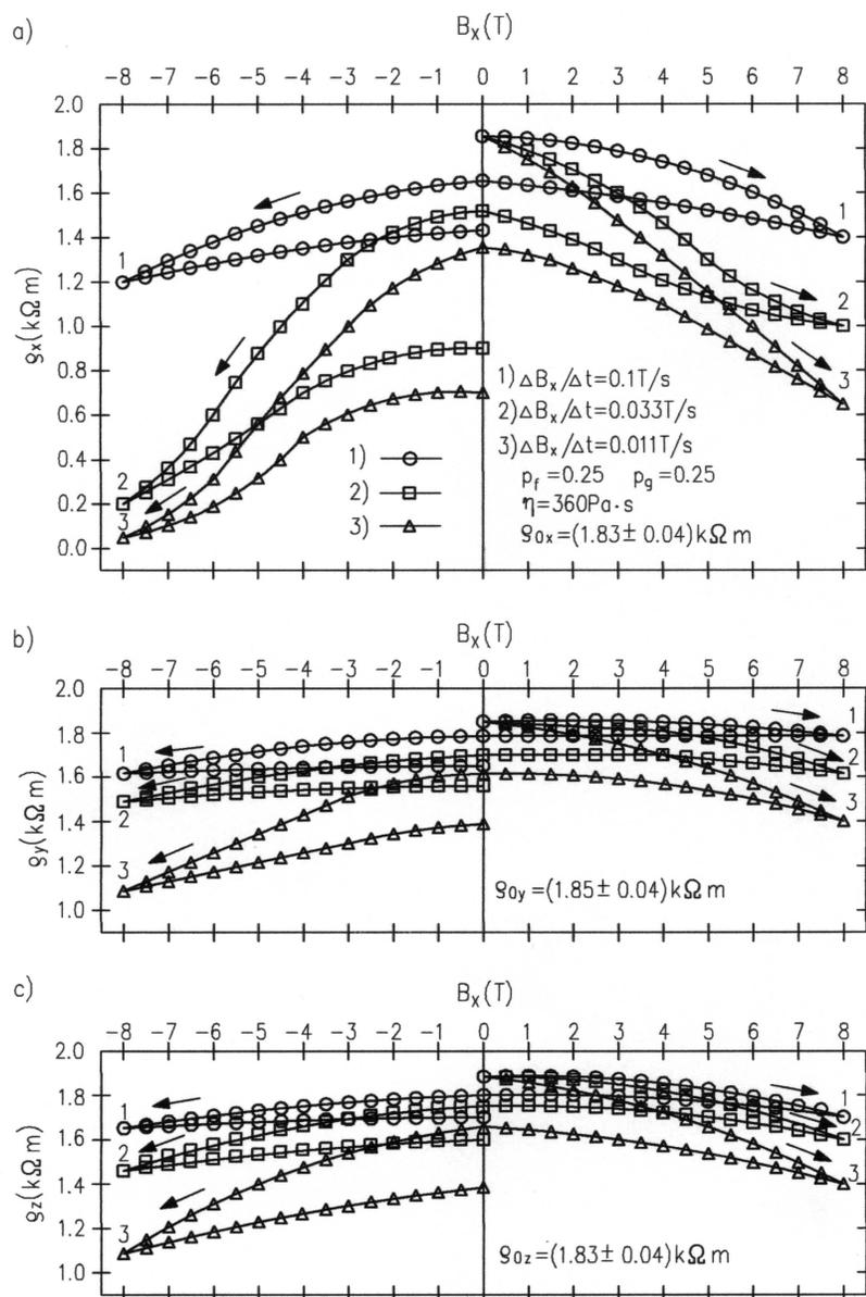
Fig. 5: Dependence of the specific resistance of the suspension sample  $\rho_x$ ,  $\rho_y$ ,  $\rho_z$  measured respectively: in directions of an  $x$ ,  $y$ ,  $z$  axis on the speed of the magnetic field induction changes  $\Delta B_x/\Delta t$  applied along the  $x$  axis.
