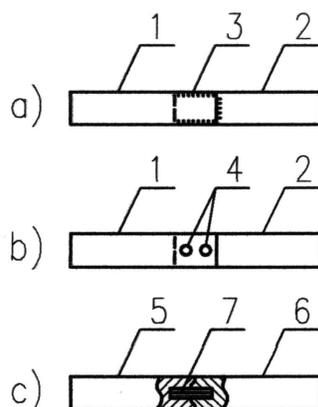
Fig. 4: Examples of method of joining the electrodes: a) soldered, b) riveted, c) twisted; 1, 2 – stripes of sheet made of different metals, 3 – soldering alloy, 4 – rivets, 5, 6 – pieces of a pipe made of different metals, 7 – screw.
