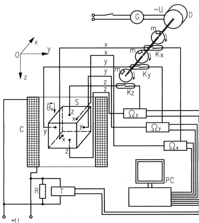
Fig. 3: Scheme of a measurement system; S – a container with sample, C – Bitter's magnet winding, T – teslameter,  $K_x$ ,  $K_y$ ,  $K_z$  – reed relay, m – neodymium magnet, d – synchronous engine, G – generator,  $Ox$ ,  $Oy$ ,  $Oz$  – ohmmeters, PC – personal computer.
