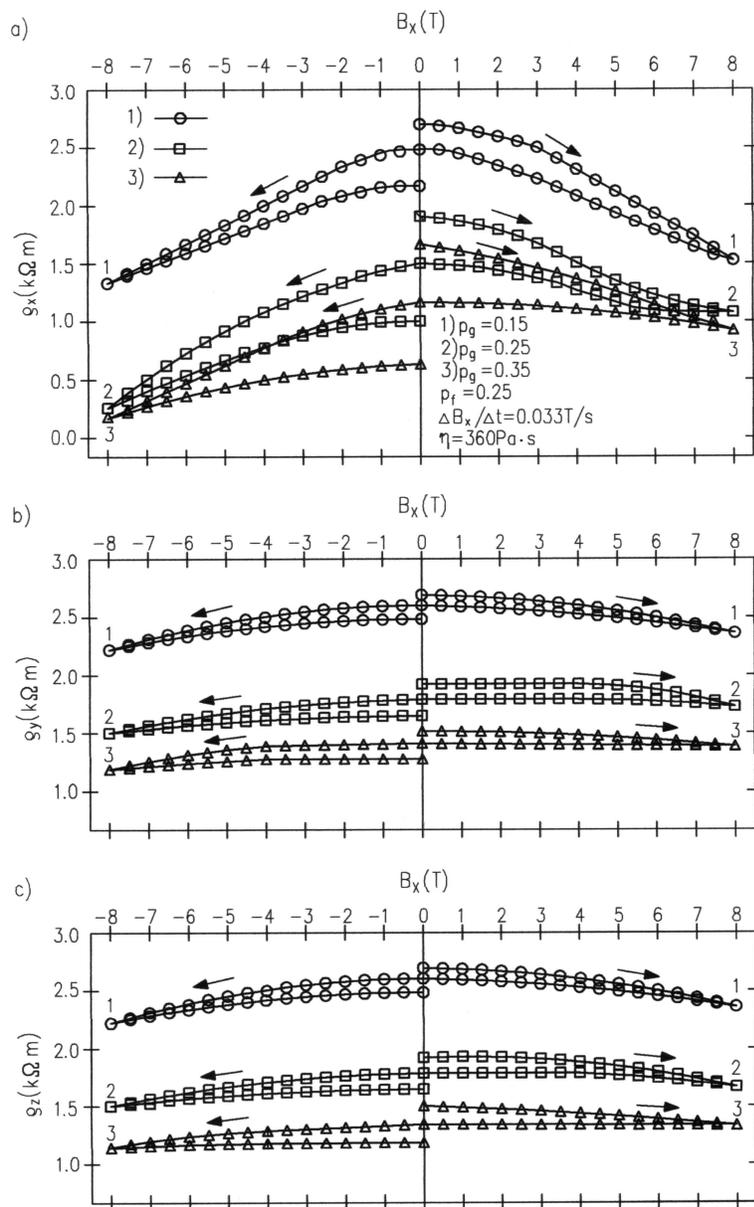
Fig. 7: Dependence of the specific resistance of the suspension sample  $\rho_x$ ,  $\rho_y$ ,  $\rho_z$  measured respectively: in directions of an  $x$ ,  $y$ ,  $z$  axis on the magnetic field induction  $B_x$ , applied along the  $x$  axis, for different factors of filling by graphite particles  $p_g$ .
