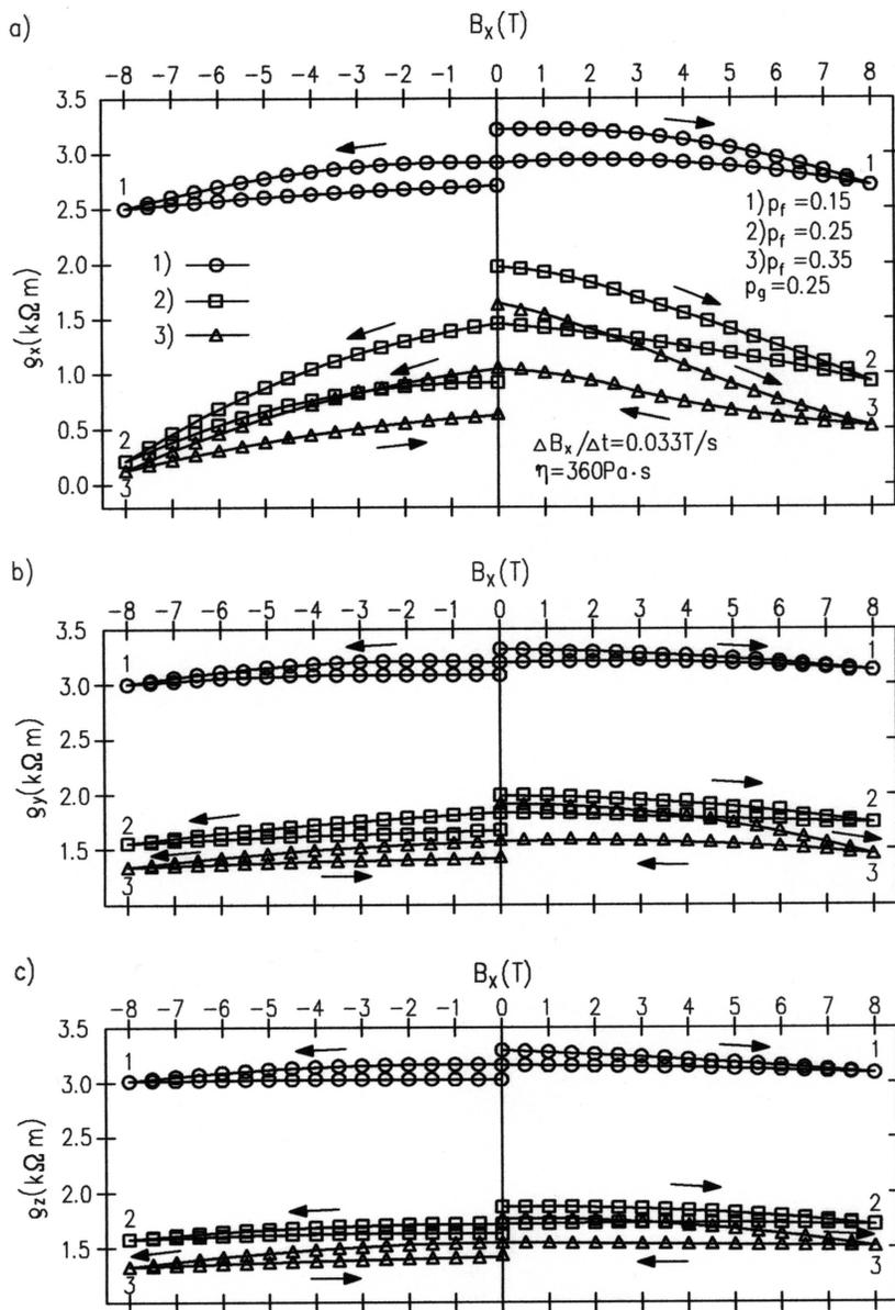
Fig. 6: Dependence of the specific resistance of the suspension sample  $\rho_x$ ,  $\rho_y$ ,  $\rho_z$  measured respectively: in directions of an  $x$ ,  $y$ ,  $z$  axis on the magnetic field induction  $B_x$ , applied along the  $x$  axis, for different factors of filling by iron particles  $p_f$ .
