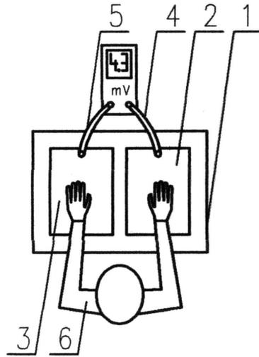
Fig. 2: “Hand battery” in the top view; 1 – insulating plate, 2, 3 – pieces of sheet made of different metals, 4, 5 – wires, 6 – a human, mV – millivoltmeter.
