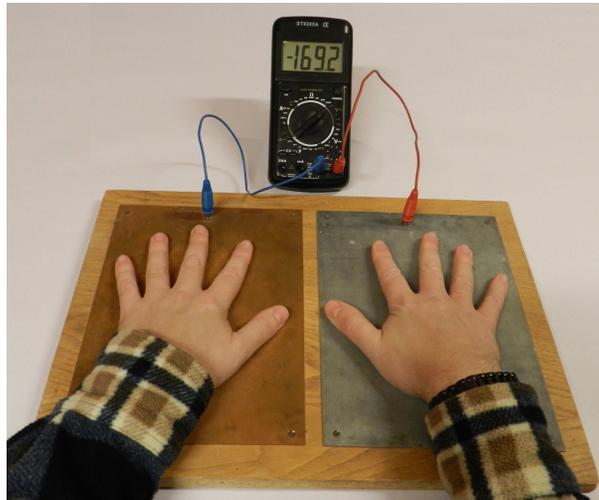
Photo 1. One of the examples of “a hand battery” in action.
