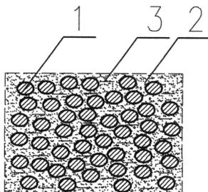
Fig. 1: Structure of suspension before applying a magnetic field; 1 – ferromagnetic particle, 2 – graphite particle, 3 – cedar wood oil.
