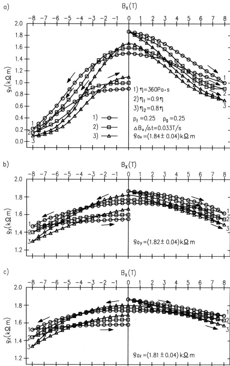
Fig. 9: Dependence of the specific resistance of the suspension sample  $\rho_x$ ,  $\rho_y$ ,  $\rho_z$  measured respectively: in directions of an  $x$ ,  $y$ ,  $z$  axis on the magnetic field induction  $B_x$ , applied along the  $x$  axis, for different coefficient viscosity  $\eta$  of disperse liquid.
