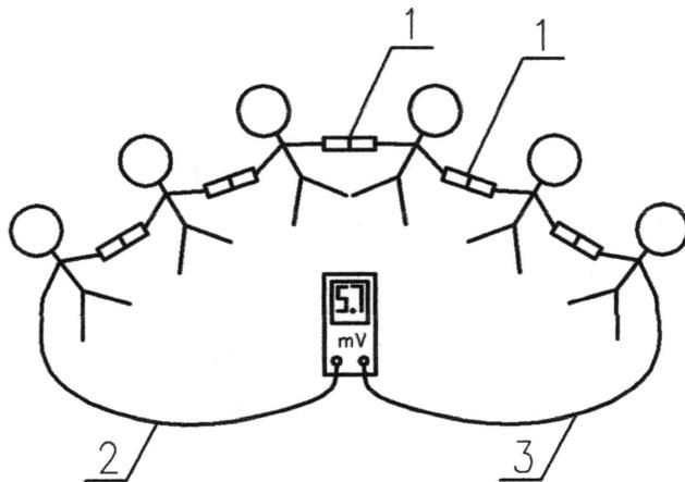
Fig. 3: Group “hand battery”; 1 – a set of electrodes, 2, 3 – wires, mV – millivoltmeter.
