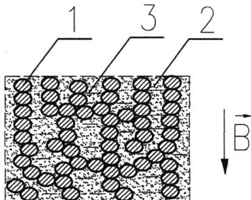
Fig. 10: Structure of the suspension after applying the magnetic field – numbers mean the same as in Fig. 1.
