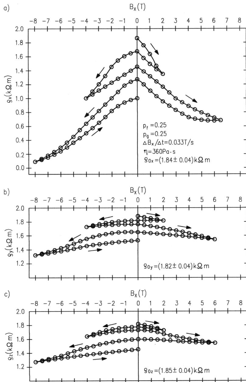
Fig. 4: Dependence of the specific resistance of the suspension sample  $\rho_x$ ,  $\rho_y$ ,  $\rho_z$  measured respectively: in directions of an  $x$ ,  $y$ ,  $z$  axis on the magnetic field induction  $B_x$ , applied along the  $x$  axis.
