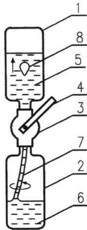
Fig. 10: Application of the universal tornado tube to investigation the Fano effect; 5, 6 – non-Newtonian fluid in the upper and lower bottle, 7 – rotating column of the fluid, 8 – air bubble, digits 1–4 determine the same elements as on Fig. 2.
