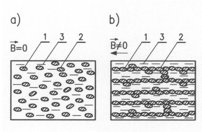
Fig. 14: Ferrofluid's structure: a) without magnetic field, b) after applying the magnetic field; 1 – magnetite's particle, 2 – a surfactant, 3 – a dispersion liquid,  $B$  – induction of the magnetic field.
