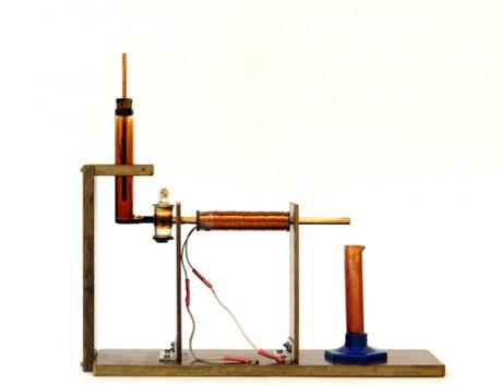
Photo 3: General view of the viscosimeter with longitudinal magnetic field and a Mariotte's bottle.
