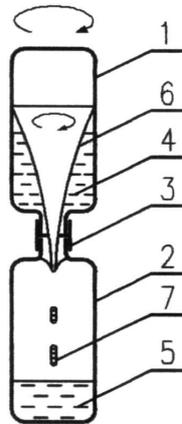
Fig. 1: Construction of the well-known tornado tube; 1, 2 – transparent plastic bottles – upper and lower one, 3 – connector, 4, 5 – water in upper and lower bottle, 6 – surface of the vortex, 7 – water flowing downwards.
