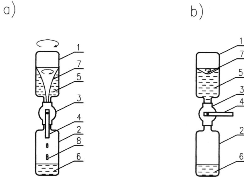
Fig. 5: Formating and dampening of the tornado in the universal tube; 5, 6 – fluid of low viscosity in the upper and lower bottle, 7 – surface of the vortex, 8 – fluid flowing downwards, digits 1–4 determine the same elements as on Fig. 2.
