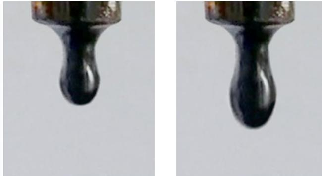
Photo 2: An example of change of shape of the ferrofluid's drop in a magnetic field: a) without the magnetic field, b) in the magnetic field of induction 60 mT.
