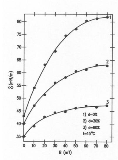
Fig. 9: Dependence of coefficients of surface tension  $\sigma$  of the ferrofluid on induction of the magnetic field  $B$  for various concentration levels  $d$  in the temperature  $t = 26^\circ\text{C}$ .
