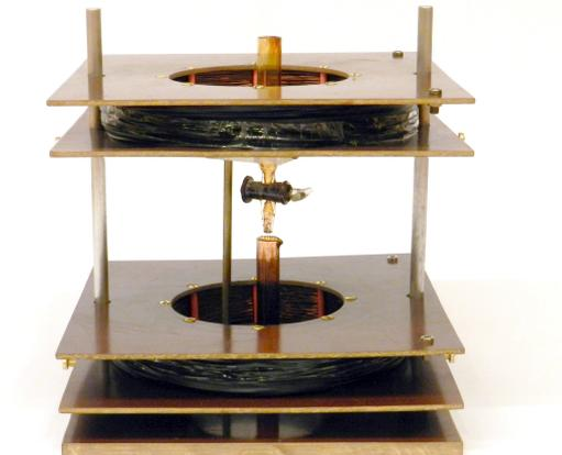
Photo 1: General view of the stalagmometer placed in Helmholtz,s coils.
