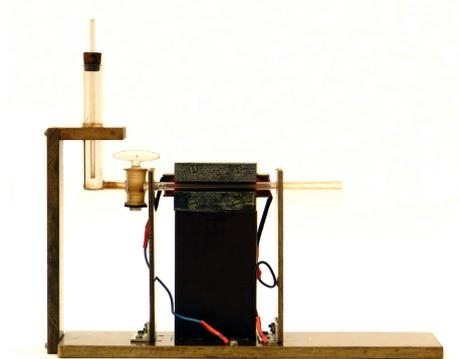
Photo 4: General view of the viscosimeter with transversal magnetic field and a Mariotte's bottle.
