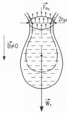
Fig. 15: Influence of the magnetic field on the change of the surface tension coefficient;  $F_{n1}$  – force of the surface tension,  $W_1$  – weight of the drop,  $r_{p1}$  – necking radius, the dashed line marks shape of the drop before applying the field,  $B$  – induction of the magnetic field.
