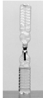
Fig. 2: Construction of the universal tornado tube; 1, 2 – transparent plastic bottles – upper and lower, 3 – body of the ball valve, 4 – lever of the ball valve.
