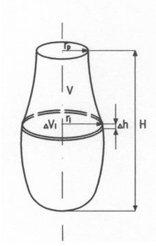
Fig. 4: A method of volume calculation of the ferrofluid's drop;  $r_i$  – layer's radius,  $\Delta h$  – layer's height,  $\Delta V_i$  – layer's volume,  $r_p$  – necking radius,  $H$  – drop's height,  $V$  – drop's volume.
