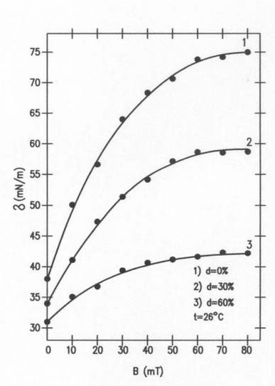
Fig. 8: Dependence of coefficients of surface tension  $\sigma$  of the ferrofluid on induction of the magnetic field  $B$  for various concentration levels  $d$  in the temperature  $t = 15^\circ\text{C}$ .
