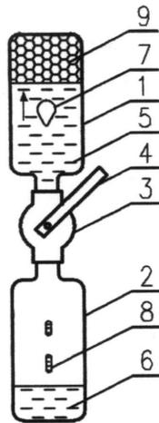
Fig. 8: Application of the universal tornado tube for investigation of foam structure and of motion in a viscous fluid; 5, 6 – shampoo in upper and lower bottle, 7 – air bubble, 8 – shampoo flowing down, 9 – foam, digits 1–4 determine the same elements as on Fig. 2.
