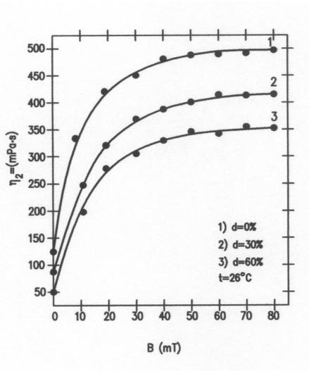
Fig. 12: Dependence of horizontal viscosity coefficients  $\eta_2$  of ferrofluid on induction of the magnetic field  $B$  for different concentration levels  $d$  in temperature  $t = 15^\circ\text{C}$ .
