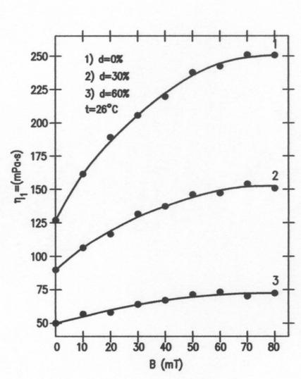
Fig. 10: Dependence of horizontal viscosity coefficients  $\eta_1$  of ferrofluid on induction of the magnetic field  $B$  for different concentration levels  $d$  in temperature  $t = 15^\circ\text{C}$ .
