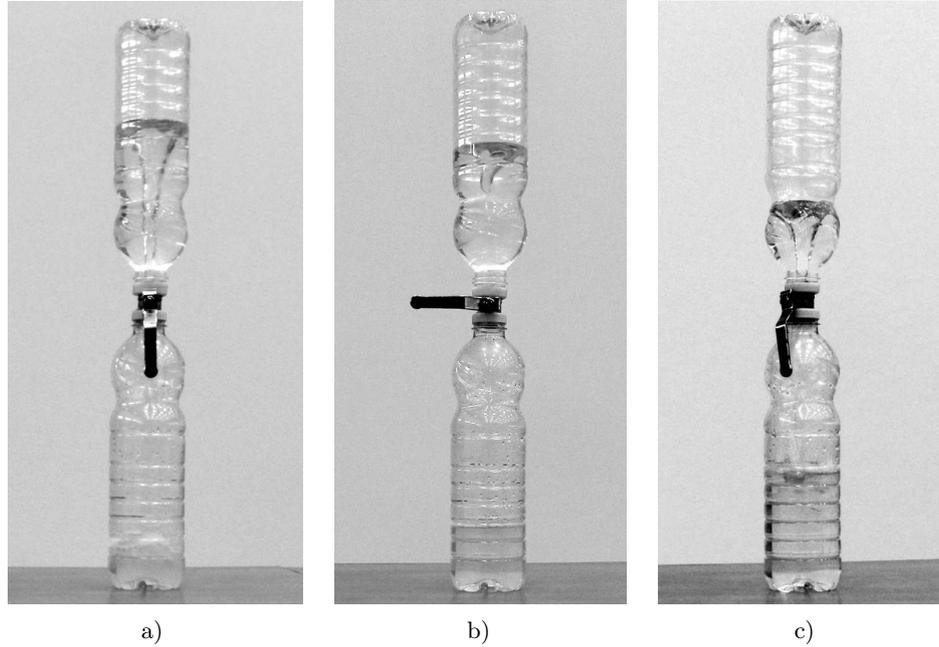
Fig. 6: Subsequent phases of tornado dampening and reanimation; a) initial tornado, b) tornado damped trough closing the valve, c) reanimated tornado.
