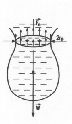
Fig. 2: Forces holding the hanging drop in balance;  $F_n$  – force of the surface tension,  $W$  – weight of the drop,  $r_p$  – necking radius.
