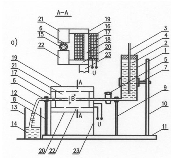
Fig. 6: Structure of a capillary viscosimeter with a transversal magnetic field and a Mariotte's bottle; numbers 1–15 – are of the same meaning as in the Fig. 5 caption, 16 – frame of coils, 17 – electromagnet's winding, 18 – electromagnet's core, 19, 20 – horizontal pole shoes, 21, 22 – vertical pole shoes, 23 – electromagnet's support,  $U$  – voltage of supply,  $B$  – induction of the magnetic field.
