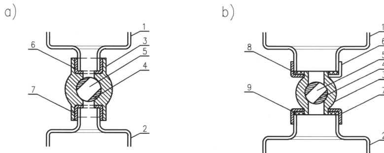
Fig. 4: Connection between the ball valve with bottles: a) with caps pushed into, b) with caps placed on, 1, 2 – transparent plastic bottles – upper and lower, 3 – body of the ball valve, 4 – ball, 5 – a hole in the ball, 6, 7 – caps of the lower and upper bottles, 8, 9 – rings.
