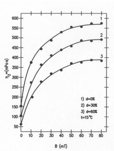
Fig. 13: Dependence of horizontal viscosity coefficients  $\eta_2$  of ferrofluid on induction of the magnetic field  $B$  for different concentration levels  $d$  in temperature  $t = 26^\circ\text{C}$ .
