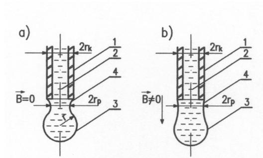
Fig. 3: Shape of the ferrofluid's drop: a) without a magnetic field, b) in a magnetic field; 1 – capillary, 2 – ferrofluid in the tube, 3 – ferrofluid's drop, 4 – necking before the drop's detachment,  $r_k$  – external radius of the capillary,  $r_p$  – necking radius,  $r$  – drop's radius,  $B$  – induction of the magnetic field.
