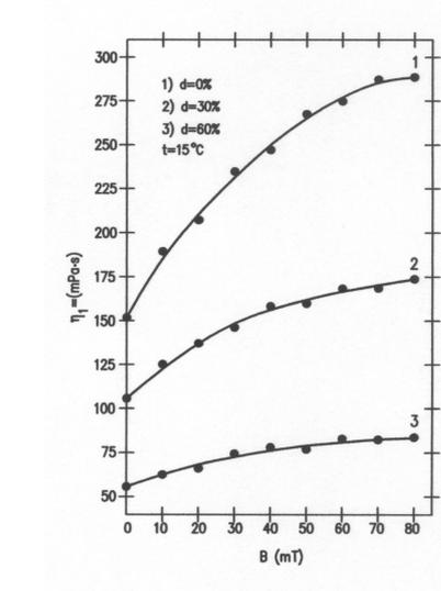
Fig. 11: Dependence of horizontal viscosity coefficients  $\eta_1$  of ferrofluid on induction of the magnetic field  $B$  for different concentration levels  $d$  in temperature  $t = 26^\circ\text{C}$ .
