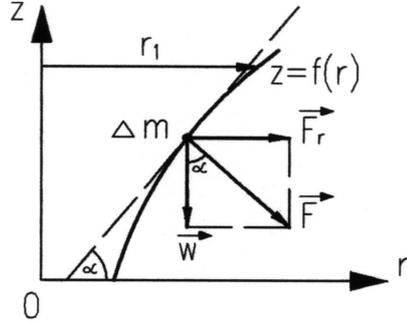
Fig. 7: Forces acting at surface of the liquid in the tornado tube;  $F_r$  – centrifugal force,  $W$  – weight,  $F$  – resultant force,  $\Delta m$  – weight of fluid element.
