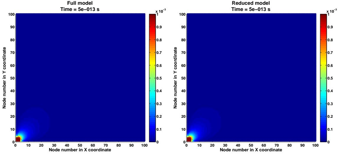
Fig. 3. The comparison of the temperature distribution inside the investigated structure described by 10000 nodes obtained using full and reduced thermal models  $500 \cdot 10^{-15}$  s after start of the simulation process.
