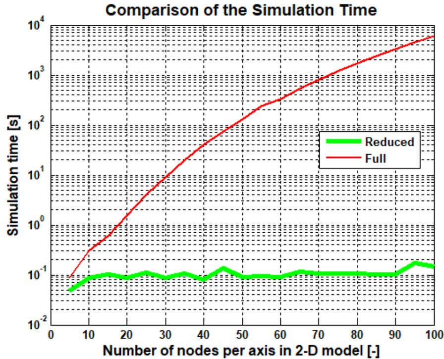
Fig. 7. The comparison of simulation times of the temperature distribution determination yielded using both full and reduced thermal models for different number of nodes.
