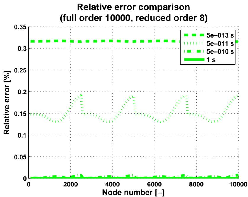
Fig. 6. The relative error analysis of the reconstruction of the full model consisting of 10000 nodes from the reduced thermal model of order 8 for some chosen time instants.
