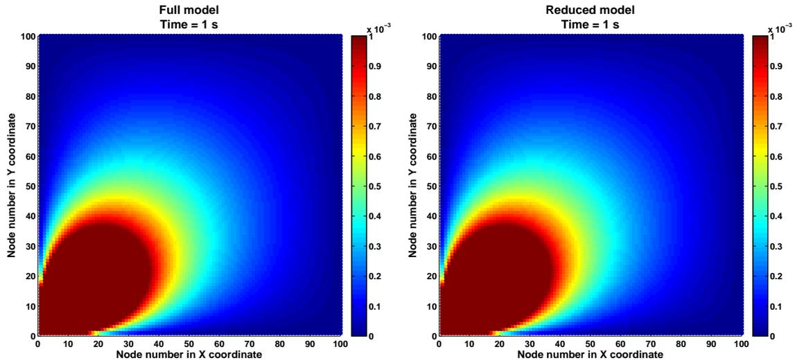
Fig. 5. The comparison of the temperature distribution inside the investigated structure described by 10000 nodes obtained using full and reduced thermal models 1s after start of the simulation process.
