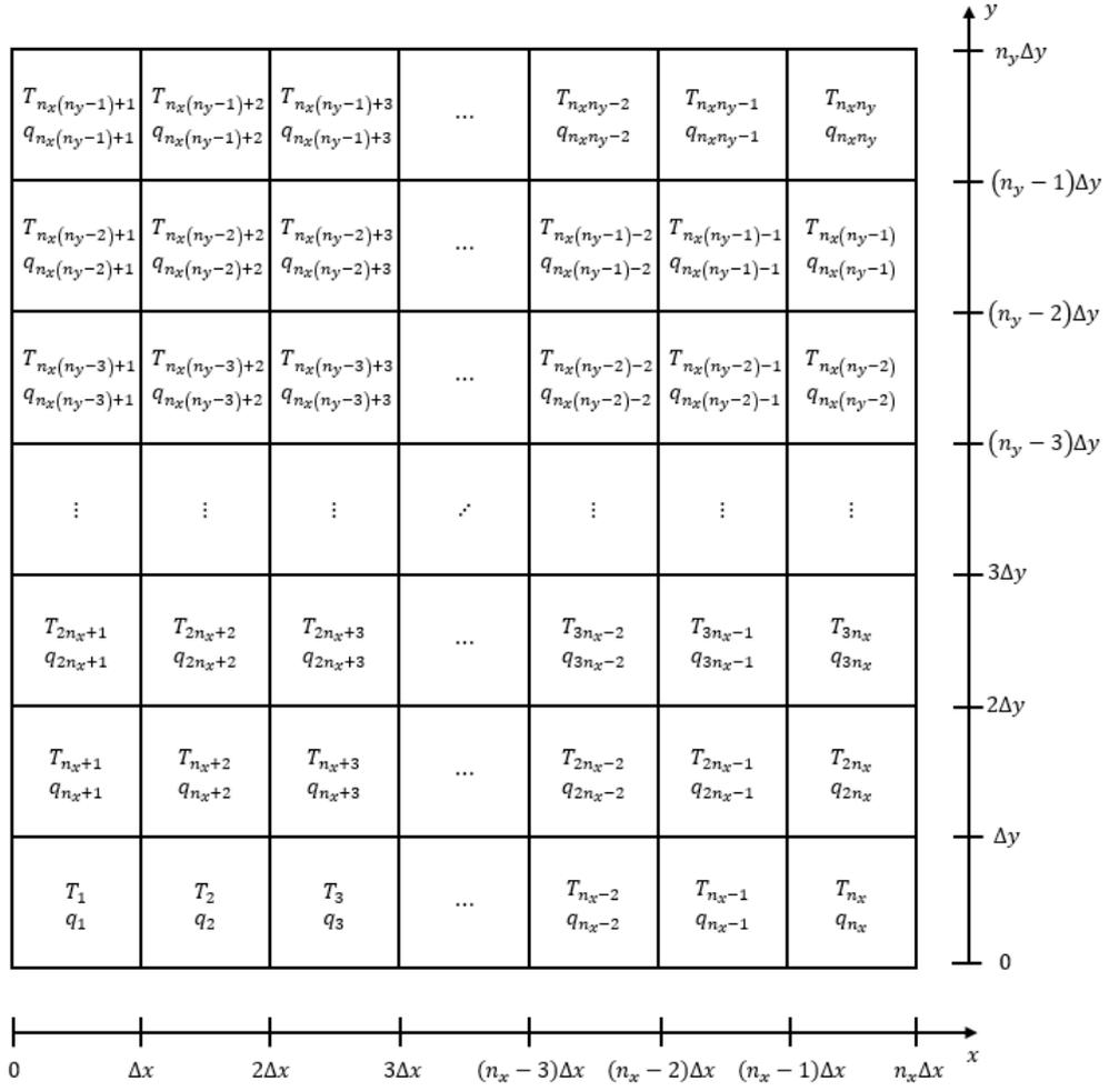
Fig. 2. The graphical representation of the discretization mesh nodes inside the structure and the way of nodes numbering process.
