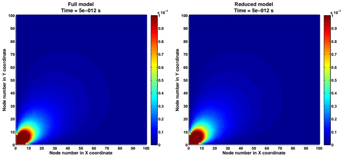
Fig. 4. The comparison of the temperature distribution inside the investigated structure described by 10000 nodes obtained using full and reduced thermal models  $5 \cdot 10^{-12}$  s after start of the simulation process.
