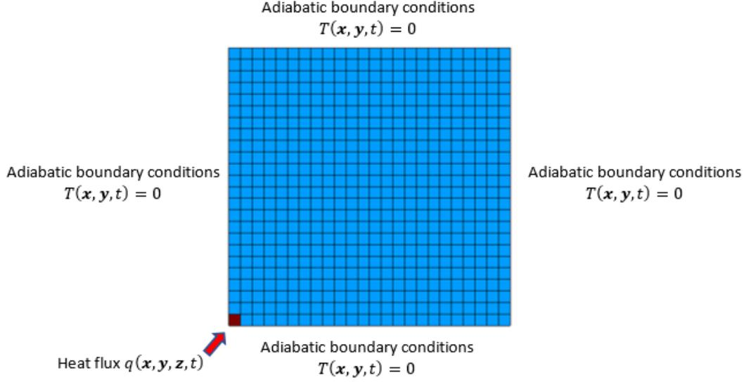
Fig. 1. The visualization of the investigated two-dimensional rectangular slab with marked adiabatic boundary conditions and direction of the heat flux.
