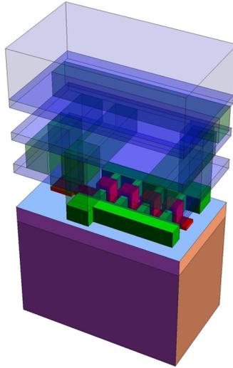
Fig. 1: Schematic 3D view of FinFET
