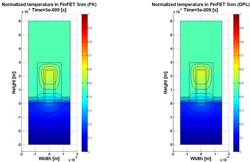
Fig. 6: The steady-state temperature distribution in 5 nm FinFET using FK and DPL models
