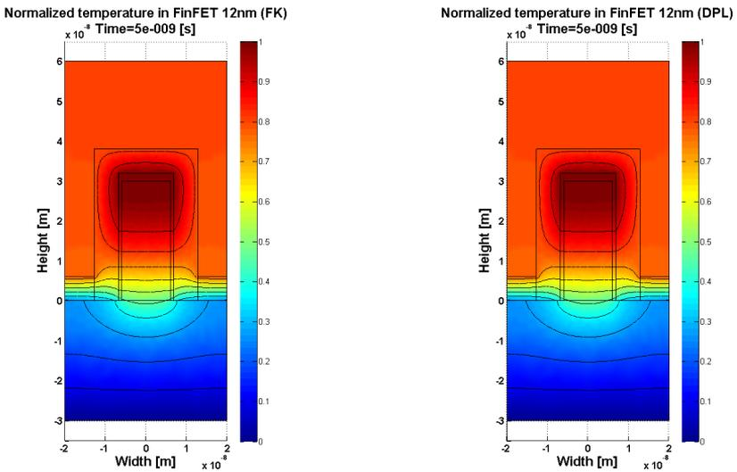
Fig. 10: The steady state temperature distribution in 12 nm FinFET using FK and DPL models
