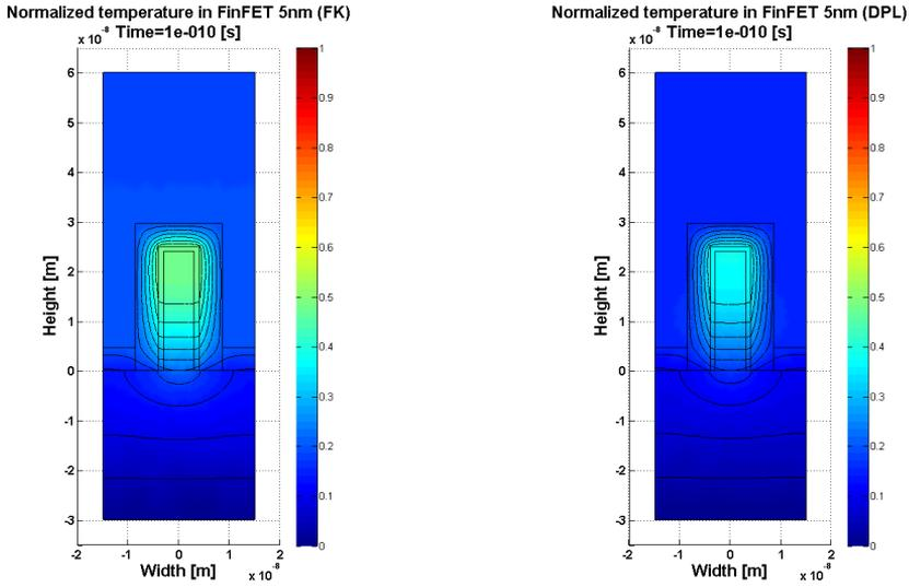
Fig. 4: The temperature distribution in 5 nm FinFET using FK and DPL models - transient analysis (part I)
