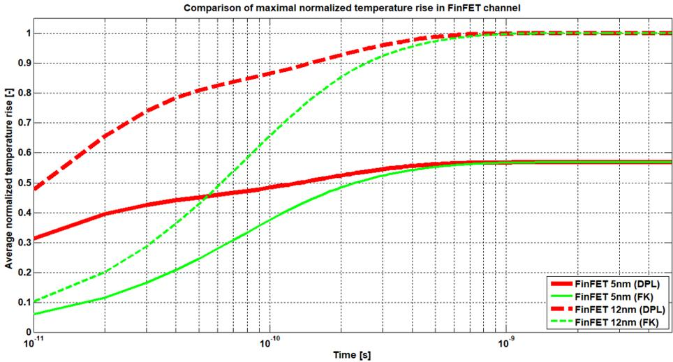
Fig. 12: Comparison of maximal normalized temperature rises obtained for 5 and 12 nm FinFETs
