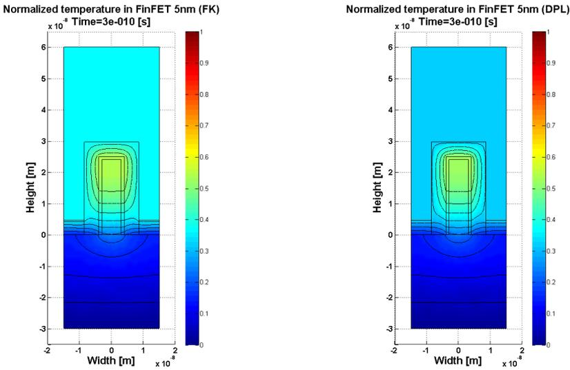
Fig. 5: The temperature distribution in 5 nm FinFET using FK and DPL models - transient analysis (part II)
