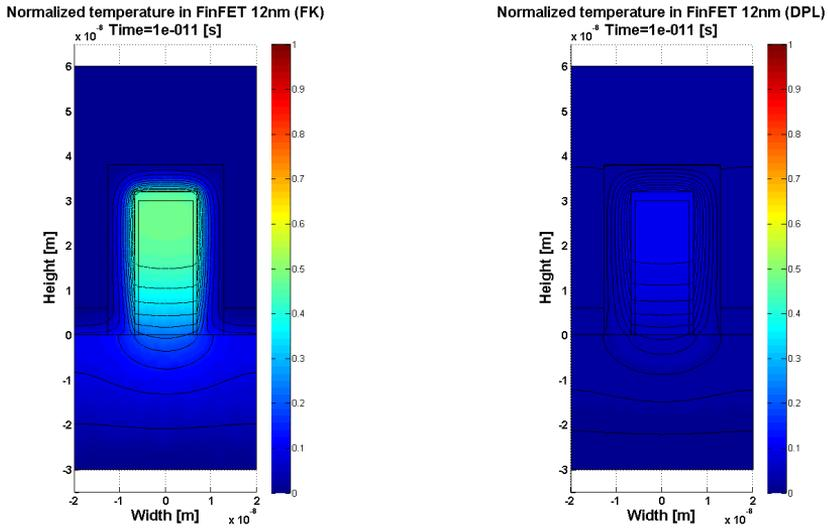
Fig. 7: The temperature distribution in 12 nm FinFET using FK and DPL models at the beginning of the simulation process
