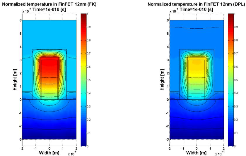
Fig. 8: The temperature distribution in 125 nm FinFET using FK and DPL models - transient analysis (part I)
