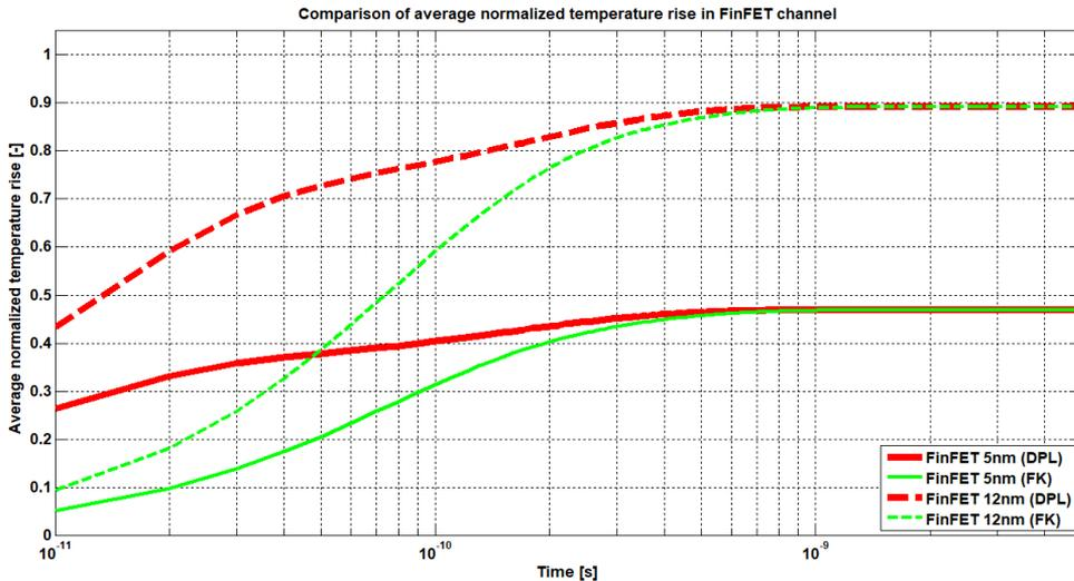
Fig. 11: Comparison of average normalized temperature rises obtained for 5 and 12 nm FinFETs
