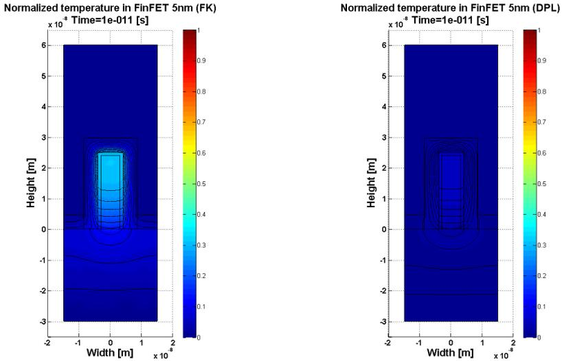
Fig. 3: The temperature distribution in 5 nm FinFET using FK and DPL models at the beginning of the simulation process
