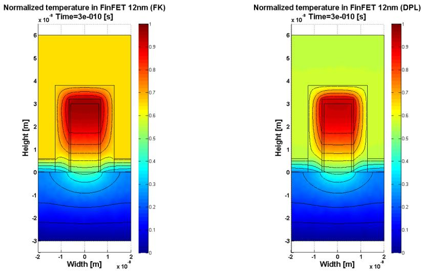
Fig. 9: The temperature distribution in 12 nm FinFET using FK and DPL models - transient analysis (part II)
