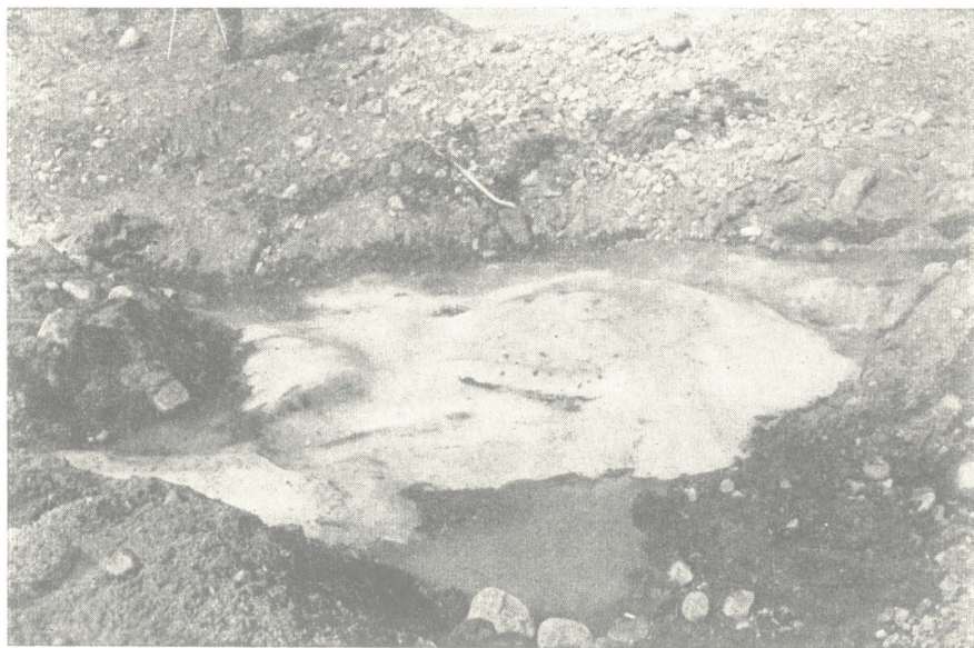
Pl. 40. Section of relict ice exposed at the permafrost table. Note convex form, with surface dipping beneath frozen gravel at the edges
