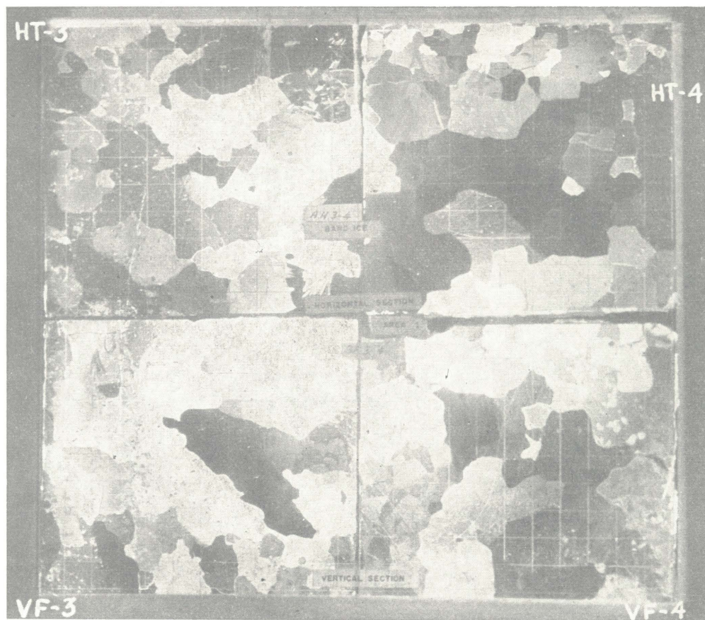
Pl. 49. Top horizontal and corresponding vertical front thin sections from sample A-13 to show variation in crystal size and form across a contact of wedge ice (HT-1, VF-1) with relict ice (HT-4, VF-)
