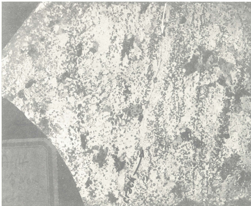
Pl. 37. Thin section of wedge ice under crossed polaroids showing fine thermal contraction crack. Thickness of section is 2 to 4 mm. Section too thick to show crystal size and shape adequately
