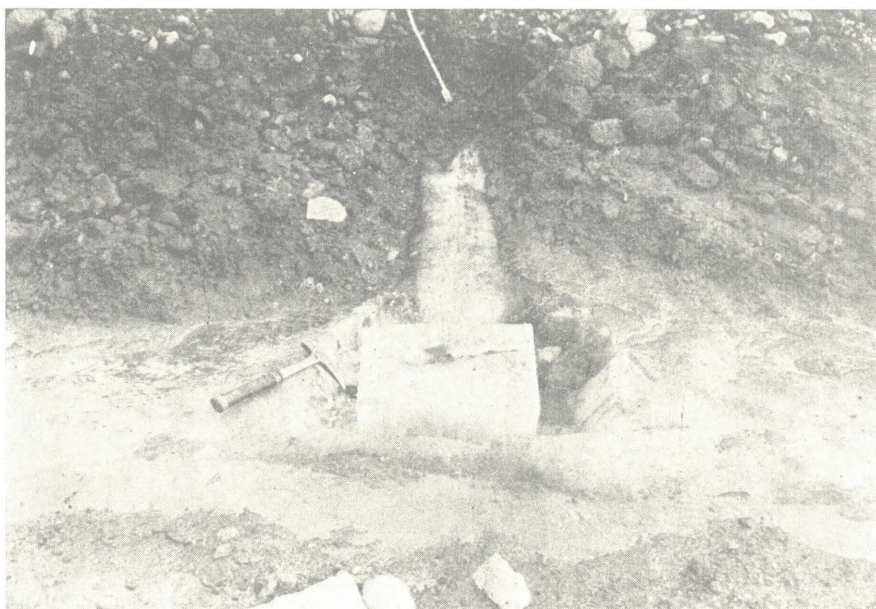
Pl. 65. Three-pronged junction of ice wedges, Area 3. Block excavated is sample C-1
