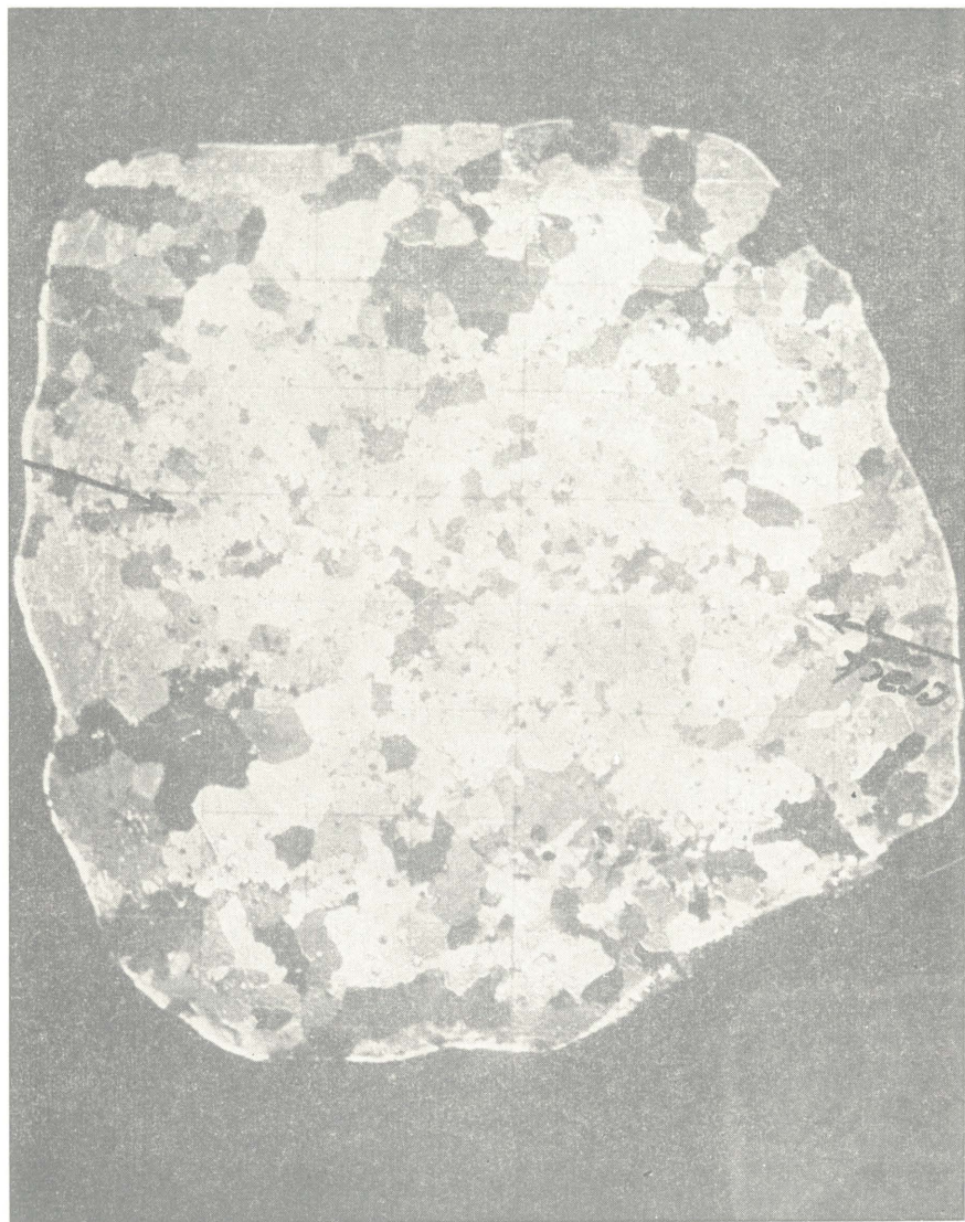
Pl. 38. Section in pl. 37 thinned to 1 mm to show variations in crystal size and shape
