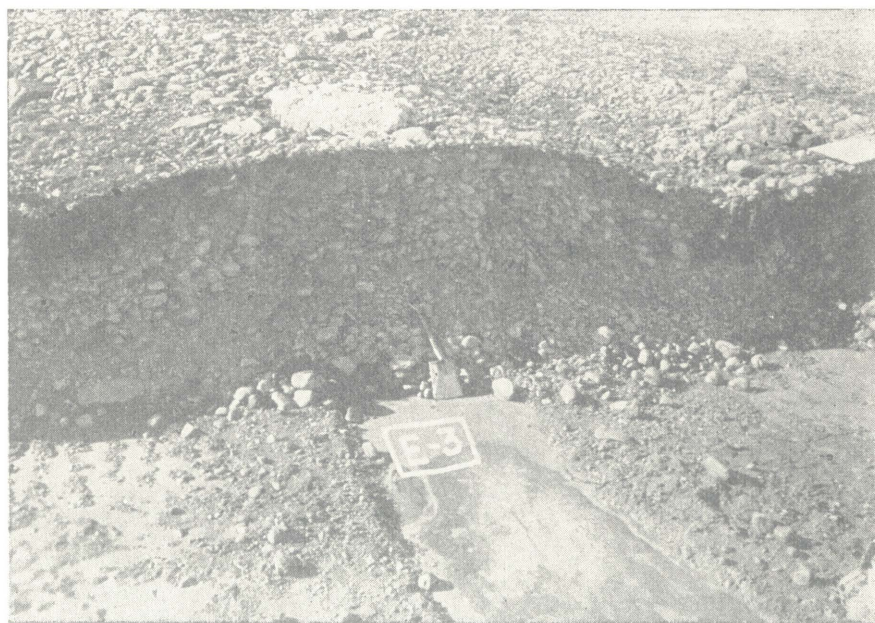
Pl. 14. Northwest wall of Area 5 trench, showing relict ice sample location and orientation of stones in the active layer
