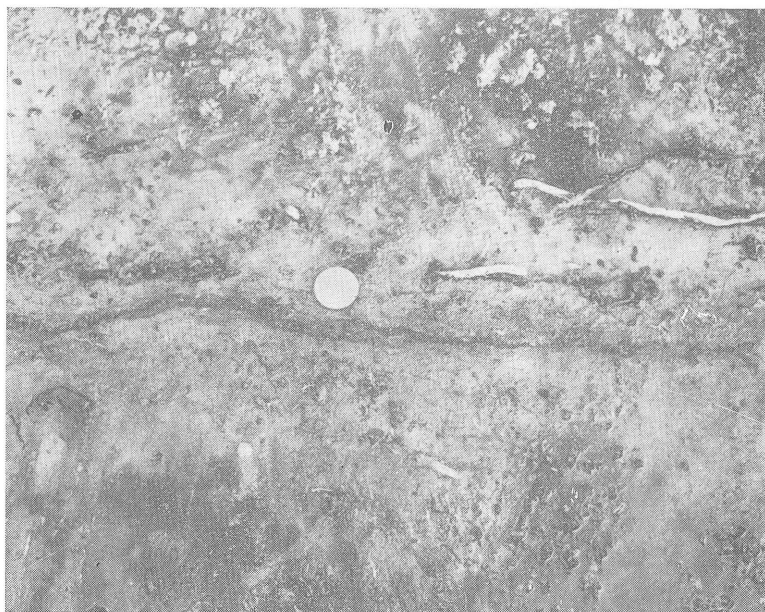
Pl. 5. View on the horizontal, frozen soil surface after the removal of the covering peat. The dark band through the picture (below the coin) is an ice vein (April 23rd, 1965)
