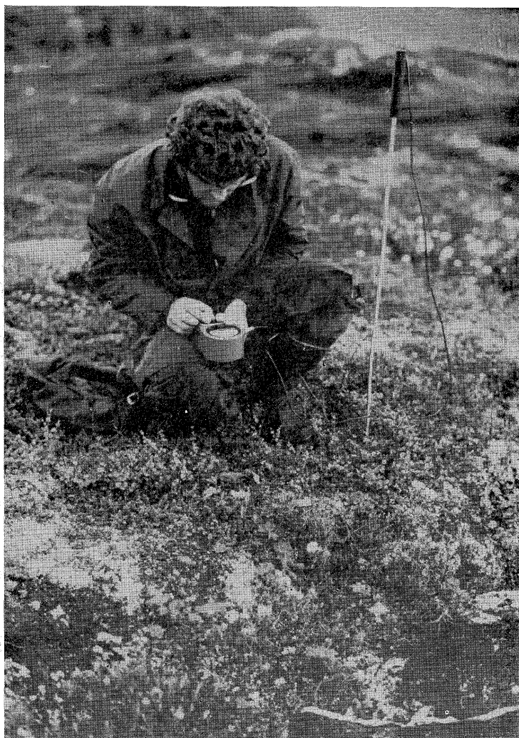
Pl. 3. Measurement of temperature inside palsa using Wallace-Thermex thermometer
