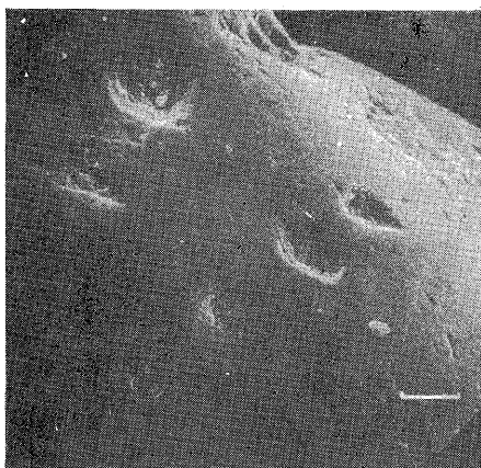
Pl. 23. Smooth grain surface with deep erosion cuts. The marked section = 25\ \mu\text{m}
