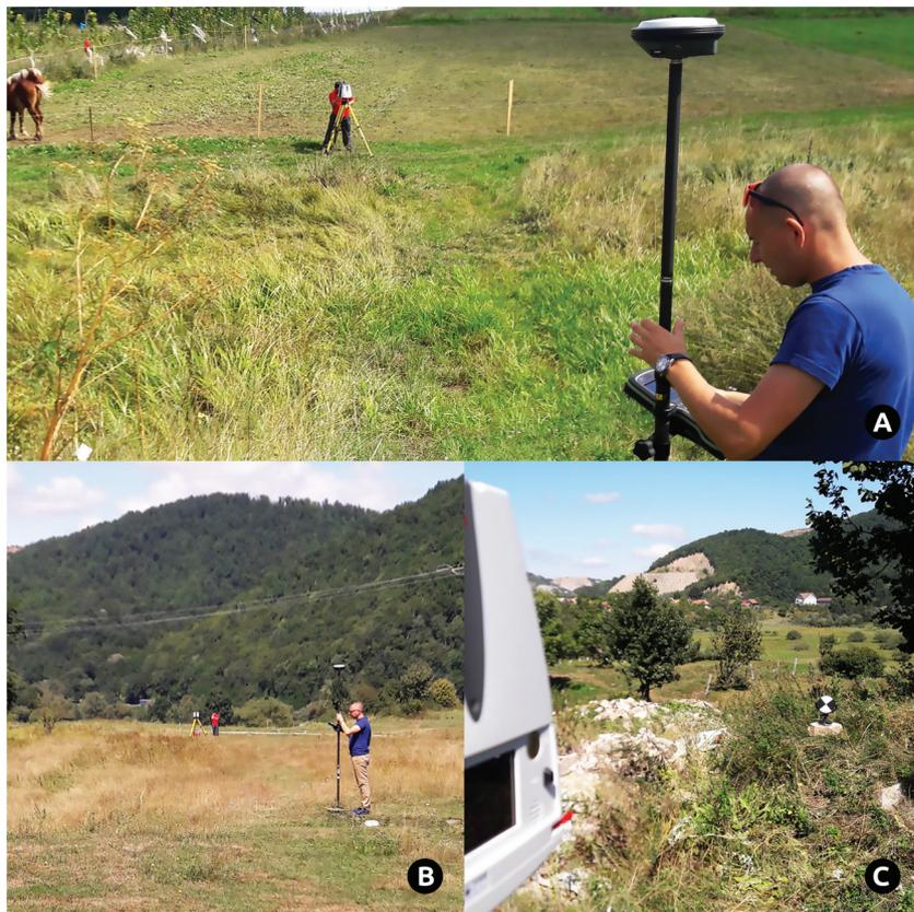
Pic. 2. Bologna, fort Resculum. HDR scanning with Leica ScanStation P50 (year 2017). A and B Establishing the geodetic network using GPS/GNNS RTK Leica Viva GS16, C – plate used as a part of the geodetic network (Photo: T. Górzynski)
