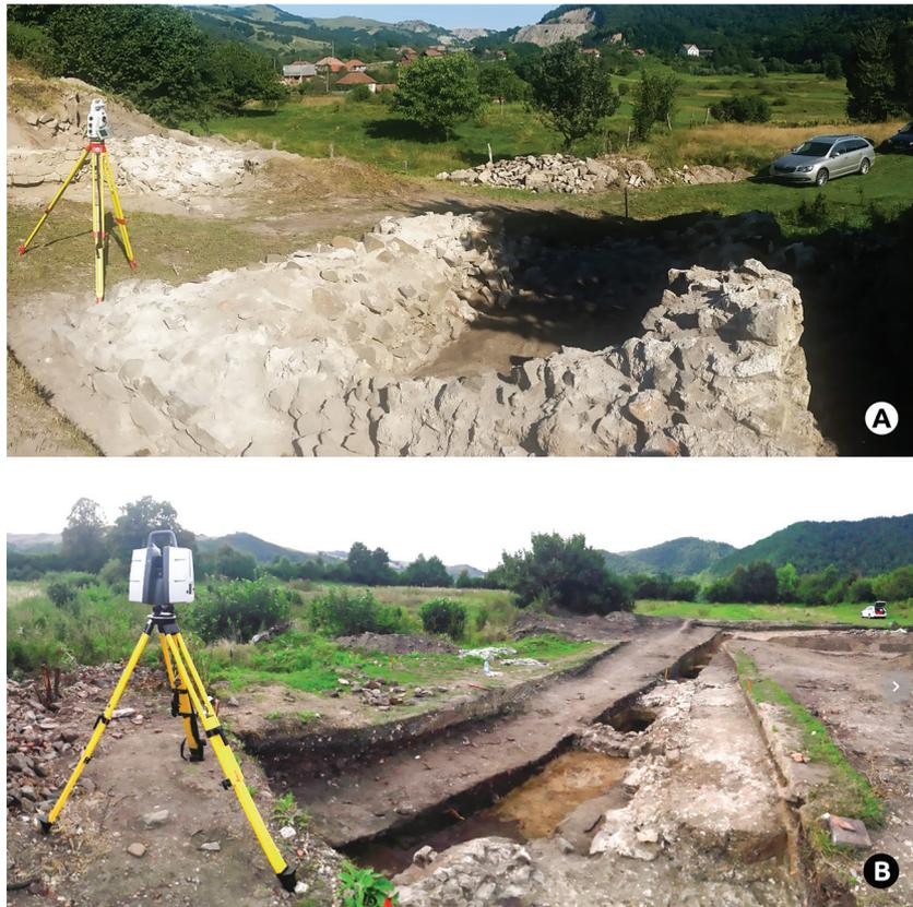
Pic. 1. Bologna, fort Resculum. Instruments used for scanning A – Leica Viva MS60 (year 2016), B – HDR Leica ScanStation P50 (year 2017) (Photo: T. Górzynski)
